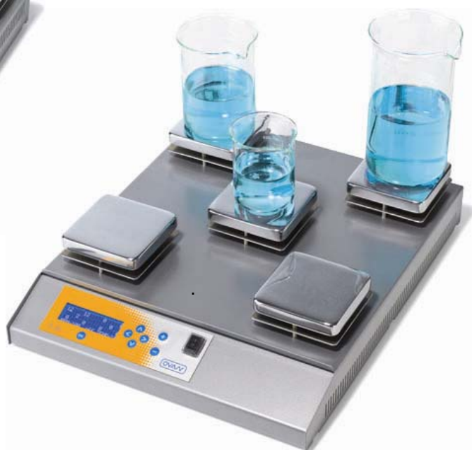
Digital hot plate multiplace, controlled by microprocessor.
